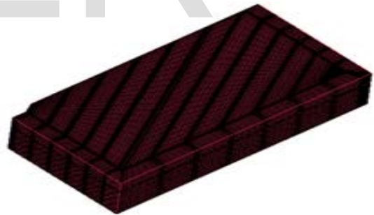
Fig-7:Premesh for half aluminum domain
